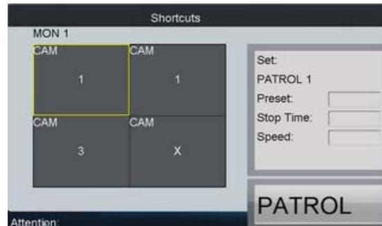
**Lock:** The *LOCK* button on the keyboard is used to lock the keyboard and mouse operation. After being locked, it is unallowable to operate all keys (except *LOCK*), joystick, mouse and the touch screen.
